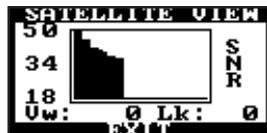
Highlight Sat Lock from the Misc Menu using the Up and Dn buttons and press Select to access the Satellite View screen.
