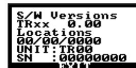
Highlight Version from the Misc Menu using the Up and Dn buttons and press Slct to open the Version window.
