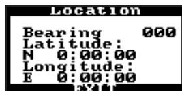
Highlight Position from the Misc Menu using the Up and Dn buttons and press Select. This will open the Location screen.
