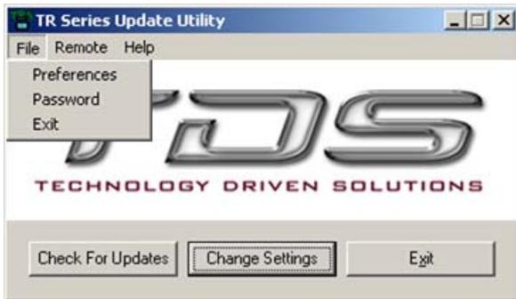
4. Select Preferences from the drop down menu to manually change the COM port that your TR head unit is connected to. However, we recommend that you leave the Auto Detect Device option checked.
