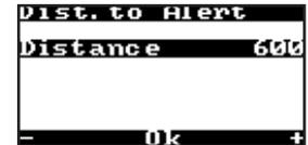
The distance to alert can be adjusted from 200 to 2,000 metres in 50m increments by using the '+' and '-' buttons and pressing Ok when ready.
