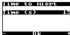
The distance to alert can be adjusted from 5 to 60 seconds in 1 sec increments by using the '+' and '-' buttons and pressing Ok when ready.
