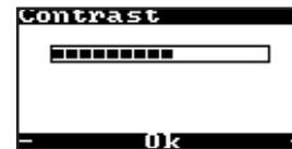
The Contrast screen will open. You can adjust using the '+' and '-' buttons and saving the setting by pressing Ok.
